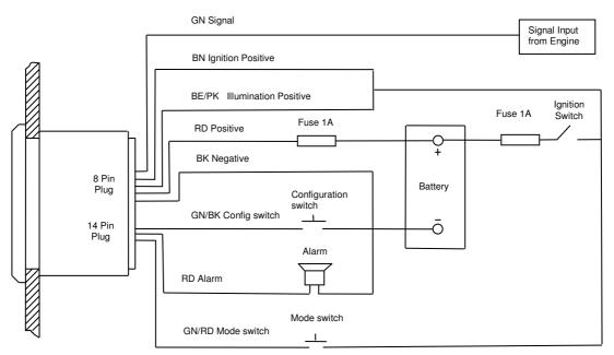
To calibrate the tacho, the number of impulses per engine revolution must be programmed into the instrument.
